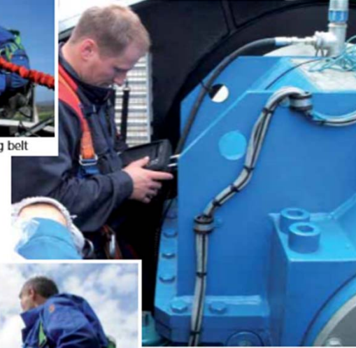
Fig. 2: Measuring the imbalance
