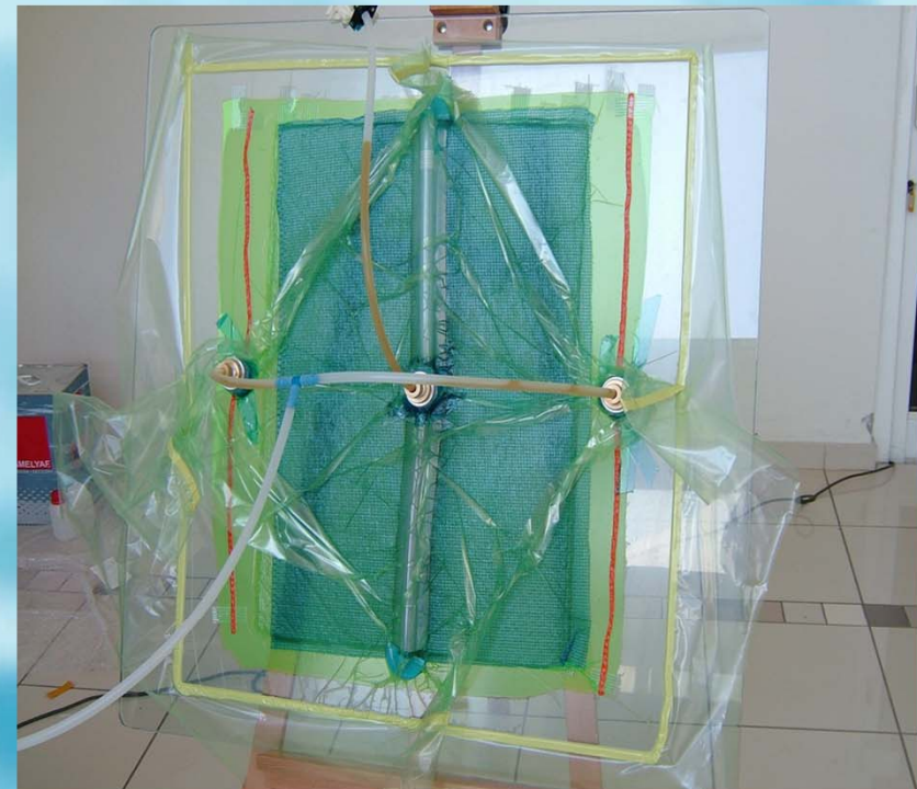
b- Pilot vacuum infusion system
