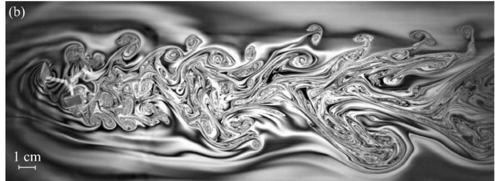
Figure 32. Soap film visualization of a clockwise rotating vertical axis wind turbine
