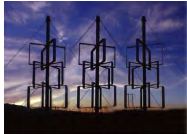
Three 530G VAVTs in Palm Springs, Calif. provide the data needed to secure the Coupled Vortex Patent.
