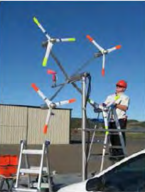
f. Four Rotor Array Wind Turbine
